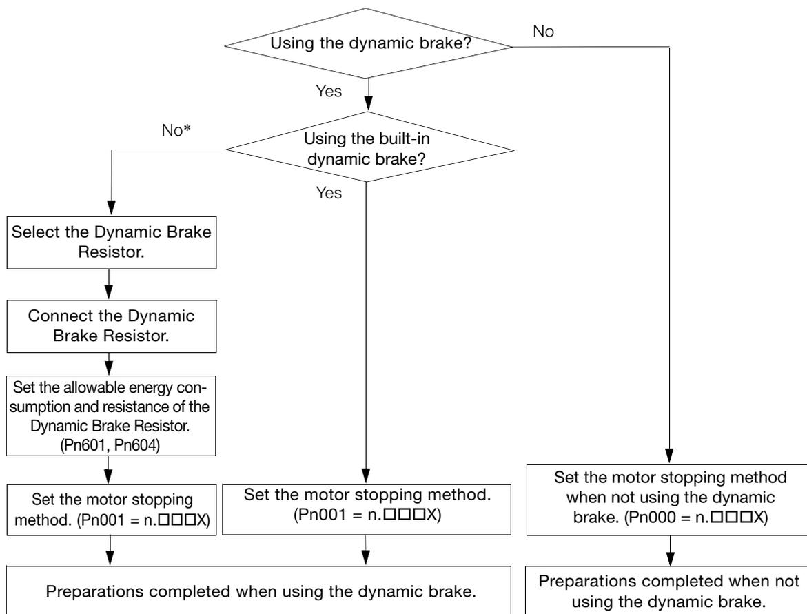
\* An External Dynamic Brake Resistor must be connected to the SERVOPACK to operate the SERVOPACK in the following manner.
