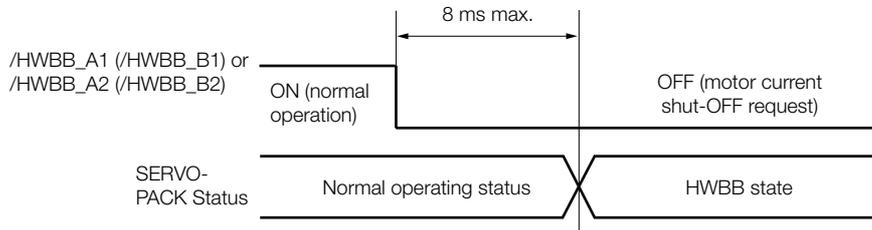
Note: 1. The OFF status is not recognized if the OFF interval of the /HWBB\_A1 or /HWBB\_A2 signal is 0.5 ms or shorter.
