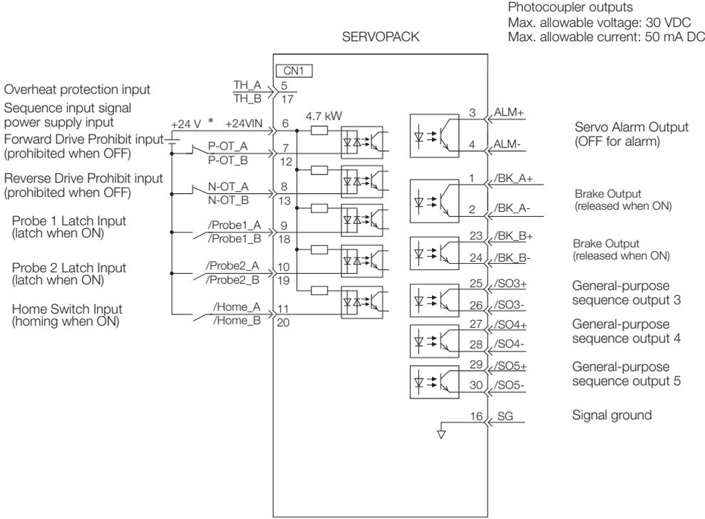
\* The 24-VDC power supply is not provided by Yaskawa. Use a 24-VDC power supply with double insulation or reinforced insulation.
