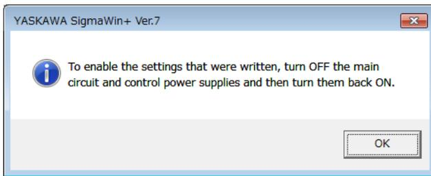
**8. To enable changes to the settings, turn the power supply to the SERVOPACK OFF and ON again.**
