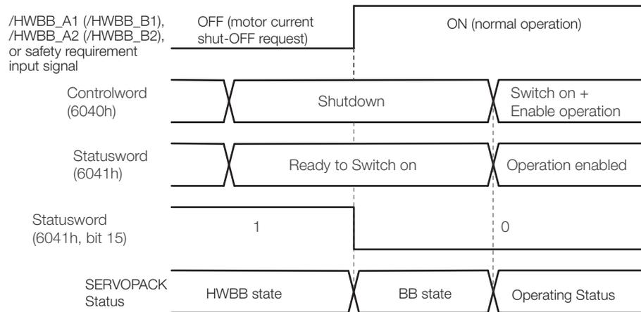
Even if the /HWBB\_A1 or /HWBB\_A2 signal is OFF and the servo ON (Enable Operation) command is received, when you turn ON the /HWBB1 and /HWBB2 signals, the SERVOPACK will enter the BB state.
