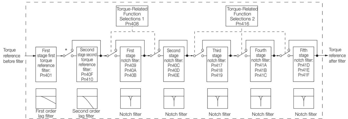
\* The second stage second torque reference filter is disabled when Pn40F is set to 5,000 (default setting) and it is enabled when Pn40F is set to a value lower than 5,000.
