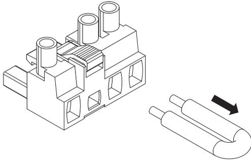
3. Remove the sheath from the wire to connect.
