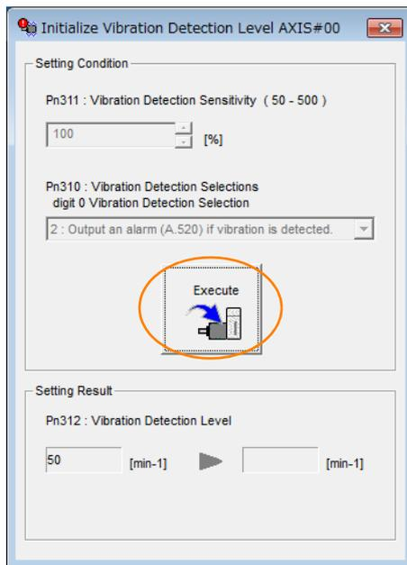
The newly set vibration detection level will be displayed and the value will be saved in the SERVO-PACK.
