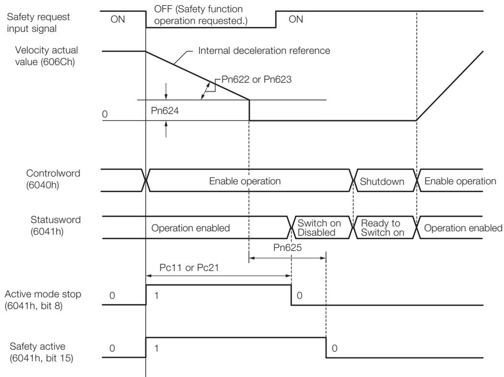
◆ When Using the SPM-D Function (Position or Speed Control)
