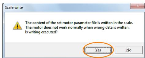
Click the **No** Button to cancel writing the motor parameters to the linear encoder. If you click the **Yes** Button, writing the motor parameter scale will start.
