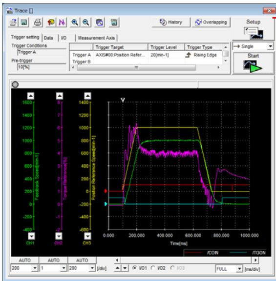
Click this button to display the Trace Setting Dialog Box shown below, and set the data to trace and the trace conditions.
