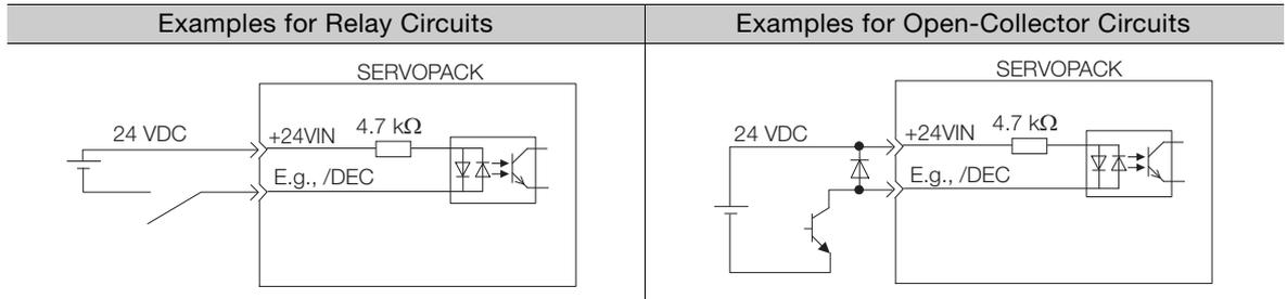
Note: The 24-VDC external power supply capacity must be 100 mA minimum.
