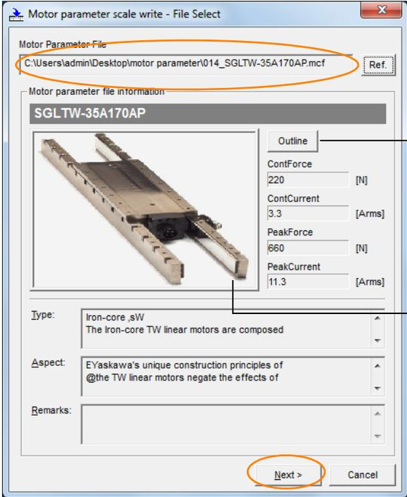
Displays an exterior view of the motor.
