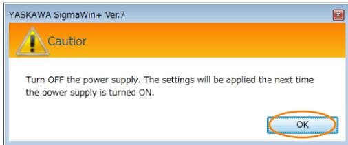
7. Turn the power supply to the SERVOPACK OFF and ON again after the SERVOPACK parameter settings have been initialized.
