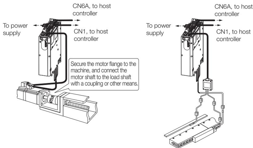
5. Turn ON the power supplies to the machine and host controller and turn ON the control power supply and main circuit power supply to the SERVOPACK.
