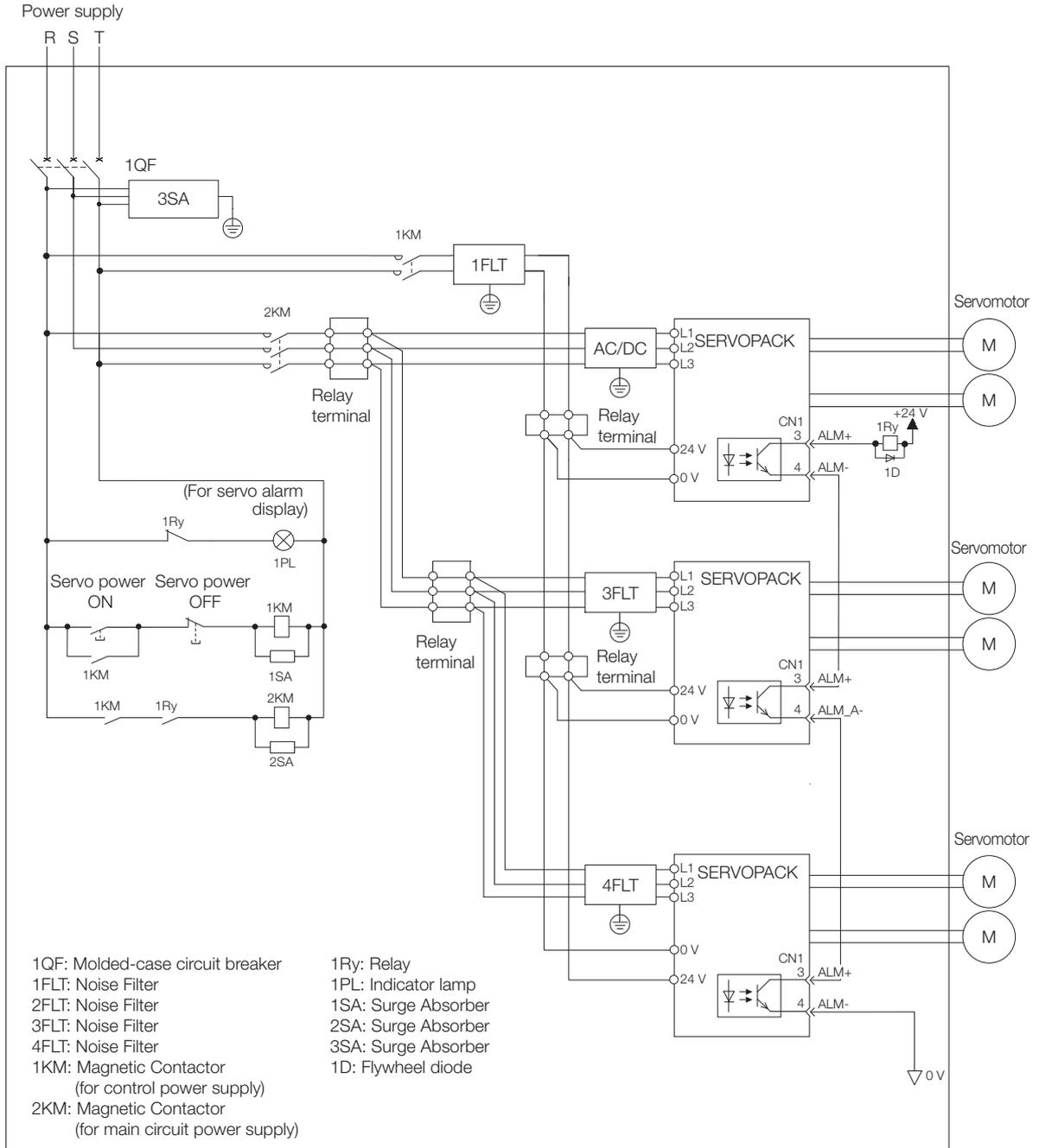
To comply with UL/cUL standards, you must install a branch circuit protective device at the power supply input section to each SERVOPACK. Refer to the following document for details.
