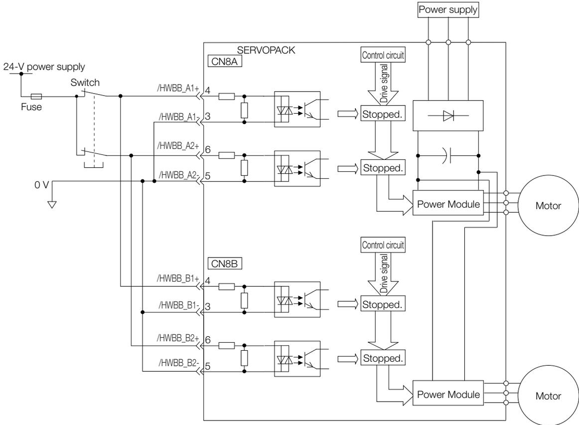
The  $\Sigma$ -7W SERVOPACKs have a HWBB for each axis.
