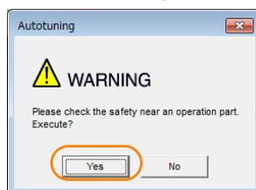
The motor will start operating and tuning will be executed. Vibration that occurs during tuning will be detected automatically and suitable settings will be made for that vibration. When the settings have been completed, the indicators for the functions that were used will light at the lower left of the dialog box.
