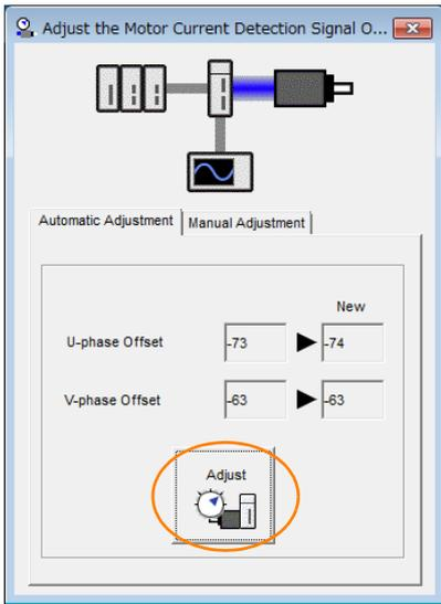
This concludes the procedure to automatically adjust the motor current detection signal offset.
