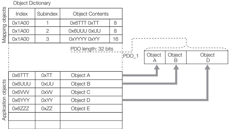
In addition to the above PDO mappings, PDOs have to be assigned to the Sync Managers to exchange EtherCAT process data. The Sync Manager PDO assignment objects (1C12h and 1C13h) establish the relationship between these PDOs and the Sync Managers.
