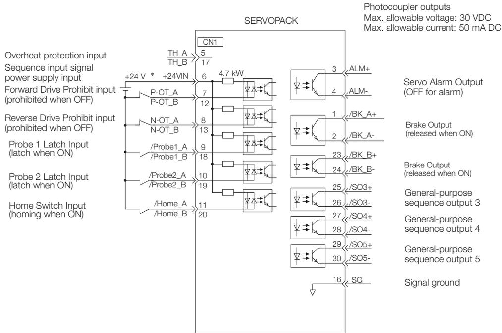
\* The 24-VDC power supply is not provided by Yaskawa. Use a 24-VDC power supply with double insulation or reinforced insulation.
