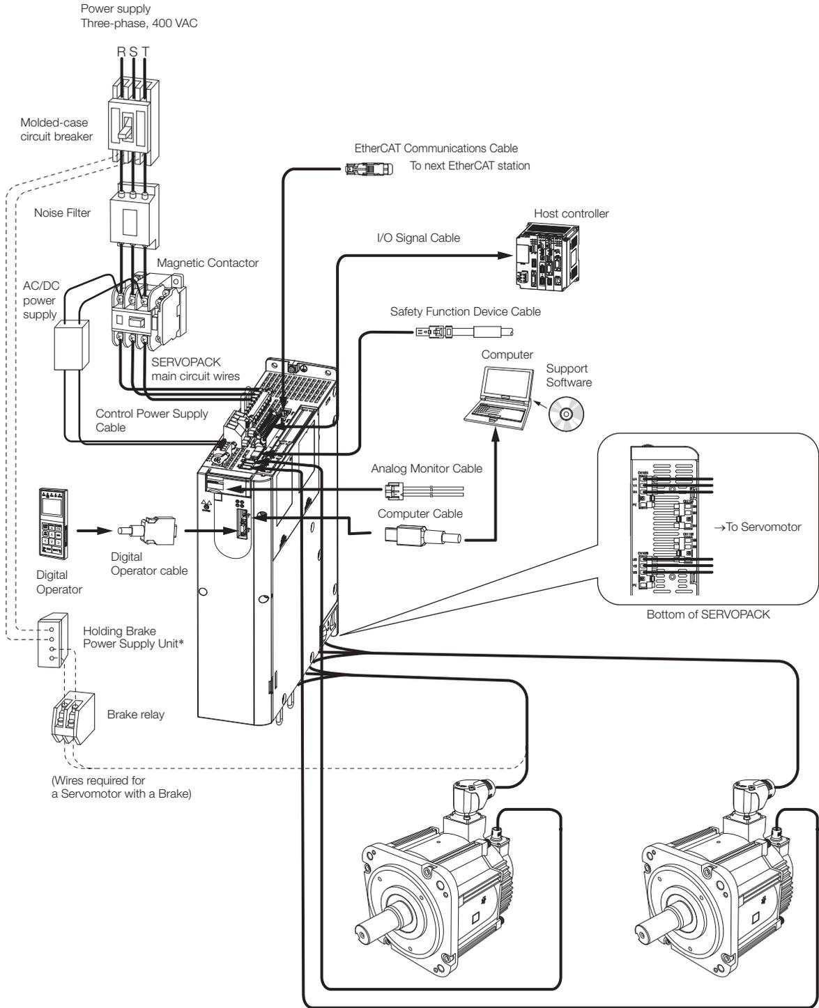
\* The power supply for the holding brake is not provided by Yaskawa. Select a power supply based on the holding brake specifications.
