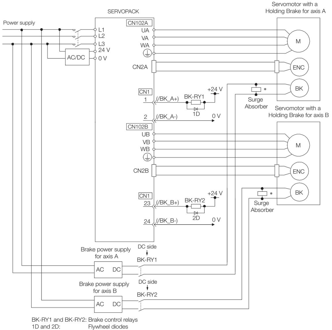
\* Install the Surge Absorber near the brake terminals on the Servomotor.
