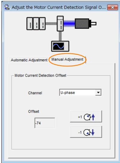
6. Set the **Channel** Box in the **Motor Current Detection Offset** Area to **U-phase**.
