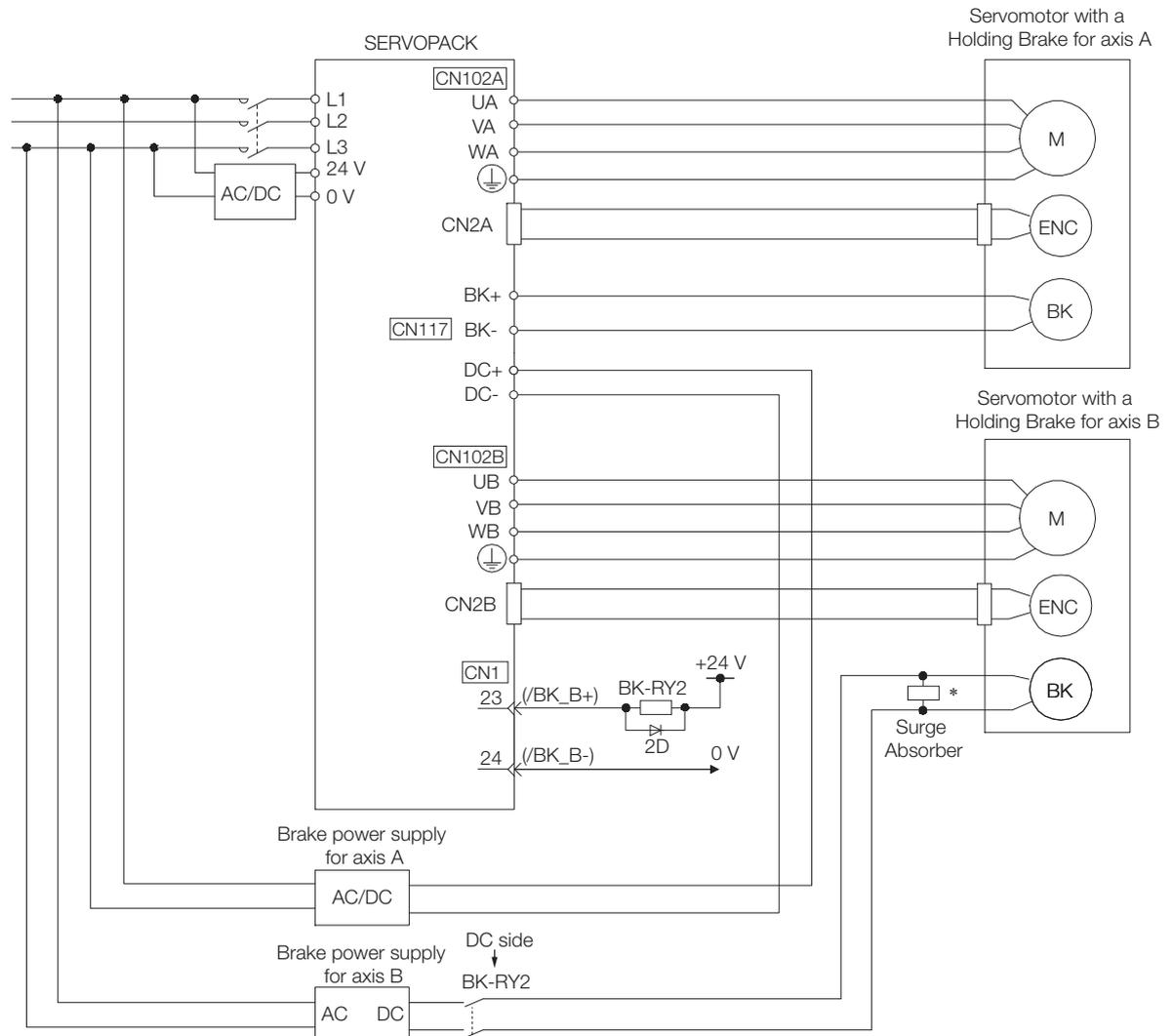
\* Install the Surge Absorber near the brake terminals on the Servomotor.
