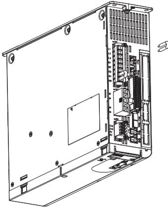
2. Connect the External Regenerative Resistor between the B1 and B2 terminals on the SERVOPACK.
