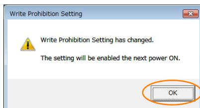
6. To enable the new setting, turn the power supply to the SERVOPACK OFF and ON again.
