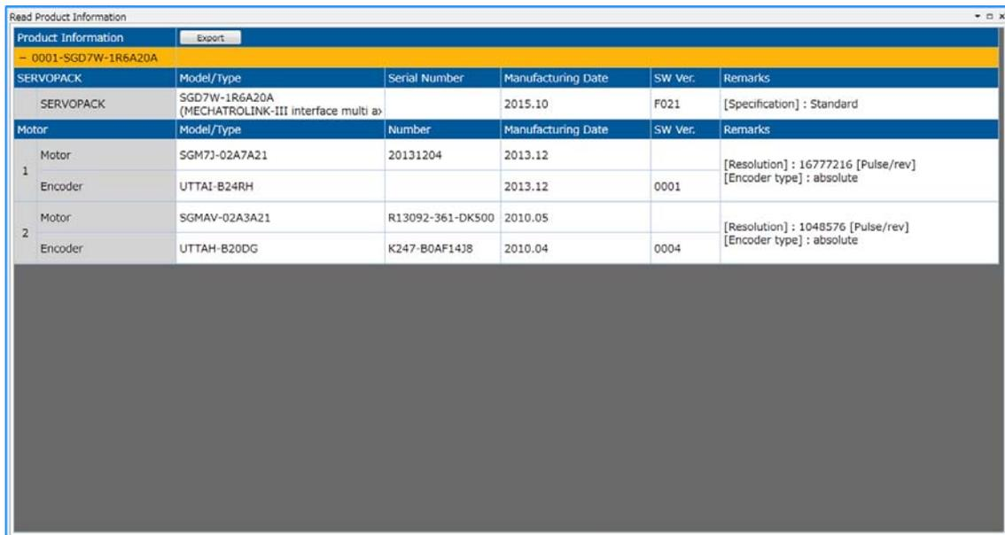
**Information** With the Digital Operator, you can use Fn011, Fn012, and Fn01E to monitor this information. Refer to the following manual for the differences in the monitor items compared with the SigmaWin+.
