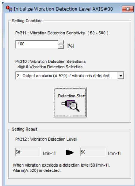
This concludes the procedure to initialize the vibration detection level.
