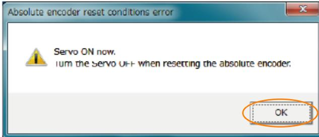
Click the **OK** Button. The Main Window will return. Turn OFF the servo and repeat the procedure from step 1.
