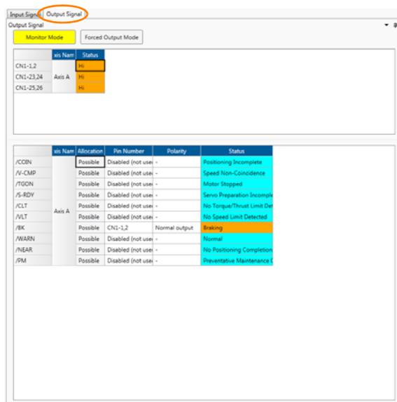
The screenshot shows the 'Output Signal' tab selected in the 'I/O Signal Allocation' window. It features 'Monitor Mode' and 'Forced Output Mode' buttons. Below are two tables: 'Output Signal' and 'Allocation Method: User allocations'. The 'Output Signal' table shows CN1-1,2, CN1-23,24, and CN1-25,26 for Axis A, all with a status of 'Hi'. The 'Allocation Method' table lists various output signals like /CCDN, /V-CMP, etc., with their allocation, pin numbers, polarities, and statuses.
