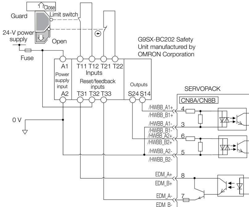
When the guard is opened, both the /HWBB\_A1 signal and /HWBB\_A2 signal turn OFF, and the EDM\_A signal turns ON. Because the feedback circuit is ON while the guard is closed, the Safety Unit is reset, the /HWBB\_A1 and /HWBB\_A2 signals turn ON, and the operation is enabled.
