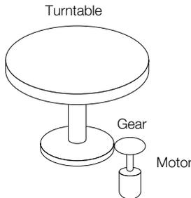
Because the turntable moves in only one direction, the upper limit to the number of rotations that can be counted by an absolute encoder will eventually be exceeded. The multiturn limit is used in cases like this to prevent fractions from being produced by the integer ratio of the number of motor rotations and the number of turntable rotations.
