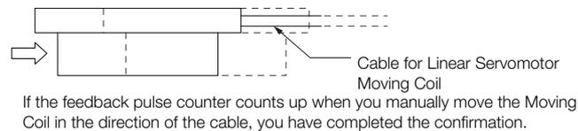
5. If the feedback pulse counter counts down, set a phase-B lead as a phase sequence of U, V, and W (Pn080 = n.□□1□) and turn the power supply OFF and ON again.
