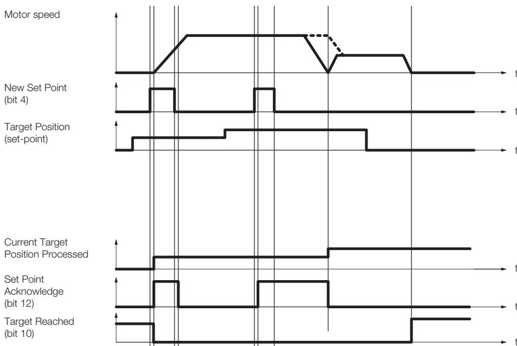
◆ SPOSING (S-curve Acceleration/Deceleration Positioning)
