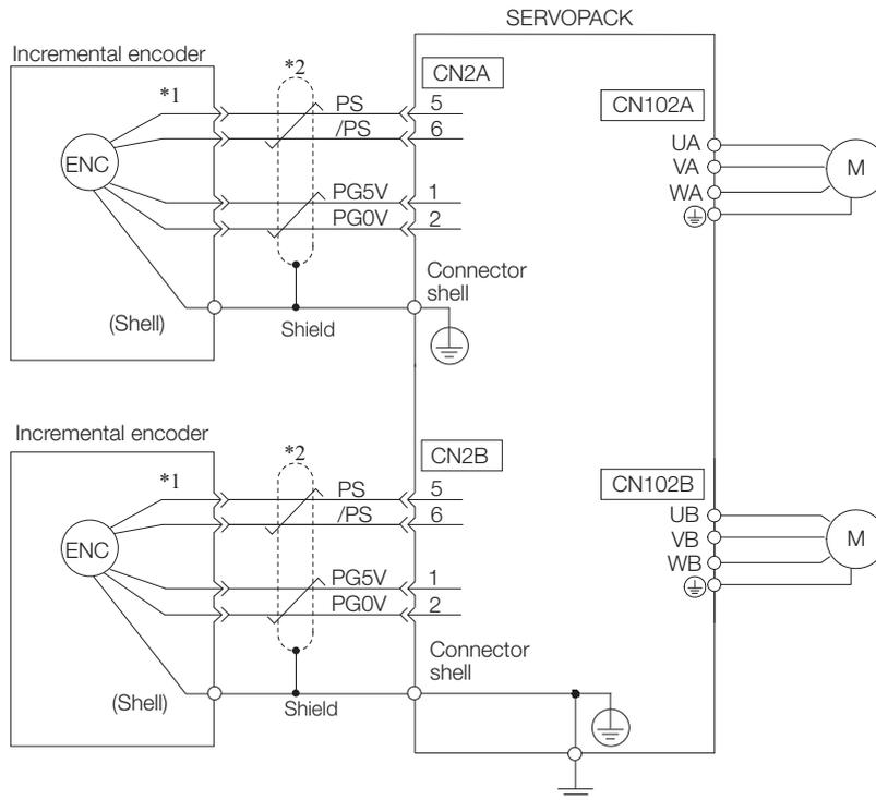
\*1. The incremental encoder pin numbers for wiring the connector depend on the Servomotor that you use.
