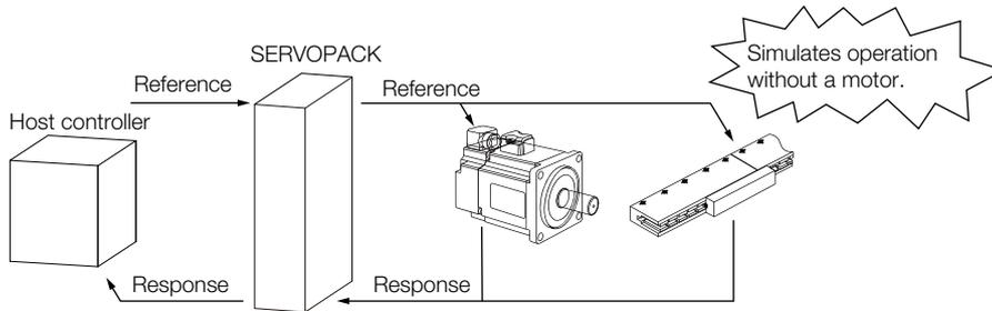
Use Pn00C = n.□□□X to enable or disable the test without a motor.
