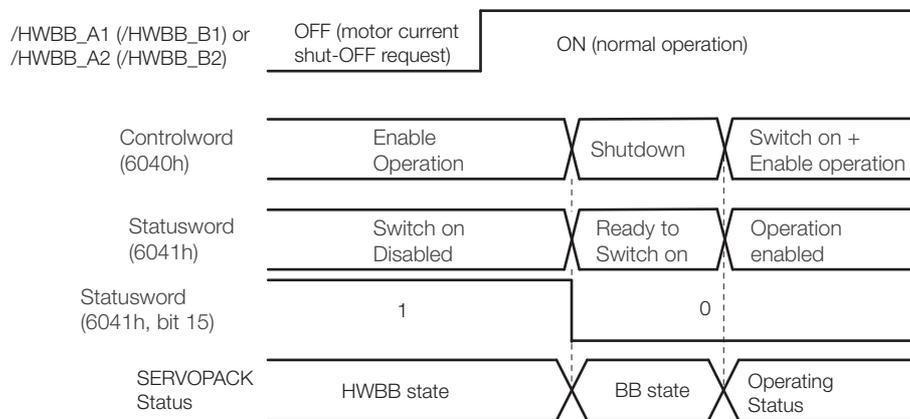
Note: If the SERVOPACK is placed in the BB state while the main circuit power supply is OFF, the HWBB state will be maintained until the Shutdown command is received.
