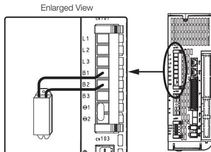
3. Set Pn600 (Regenerative Resistor Capacity) and Pn603 (Regenerative Resistor Resistance). Refer to the following section for details on the settings.
