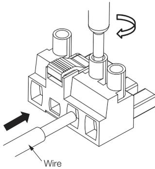
6. Connect Dynamic Brake Resistors to the D1A and D2A terminals and to the D1B and D2B terminals on the SERVOPACK.
