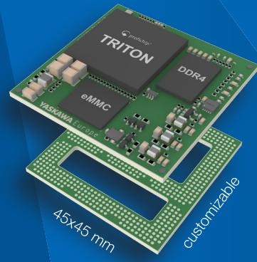
The module includes the entire processor infrastructure and comes in a compact and easy to use standard format. The additional spacer can be customized allowing adaption to alternative standards or specific customer needs.
