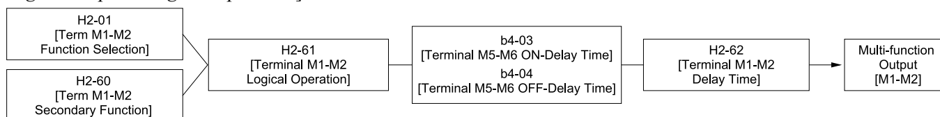
Figure 11.57 Functional Block Diagram of Logical Operation Output for MFDO 1
