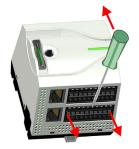
**8.** Remove the connectors, which are not necessary at the CPU.
