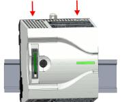
Plug the CPU from the top onto the mounting rail and turn the CPU downward until it rests on the mounting rail.
