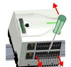
By means of a screwdriver there is the possibility to remove the connectors e.g. for module exchange with a fix wiring. For this each connector has indentations for unlocking at the top. Unlocking takes place by the following proceeding:
