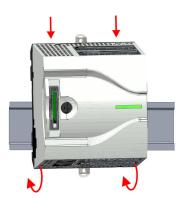
3. Plug the CPU from the top onto the mounting rail and turn the CPU downward until it rests on the mounting rail.
