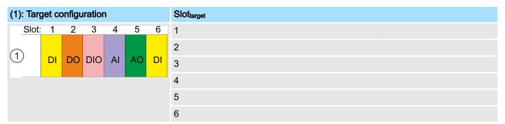
Slot<sub>target</sub> The mapping always refers to the slot of the target configuration.
