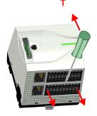
7. Remove the connectors, which are not necessary at the CPU.
