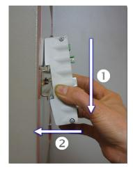
Pull-down the T1 and push it on the DIN rail.
