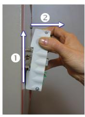
Push-up the T1 and pull it of the DIN rail.
