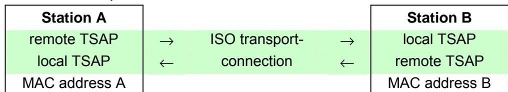
The TSAPs of an ISO transport connection must match as follows:
