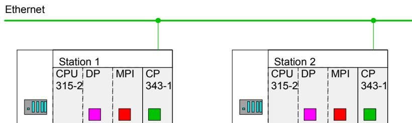
To configure the connection open the connection list. For this you choose the CPU of Station 1 and call *Insert new connection* via the context menu:
