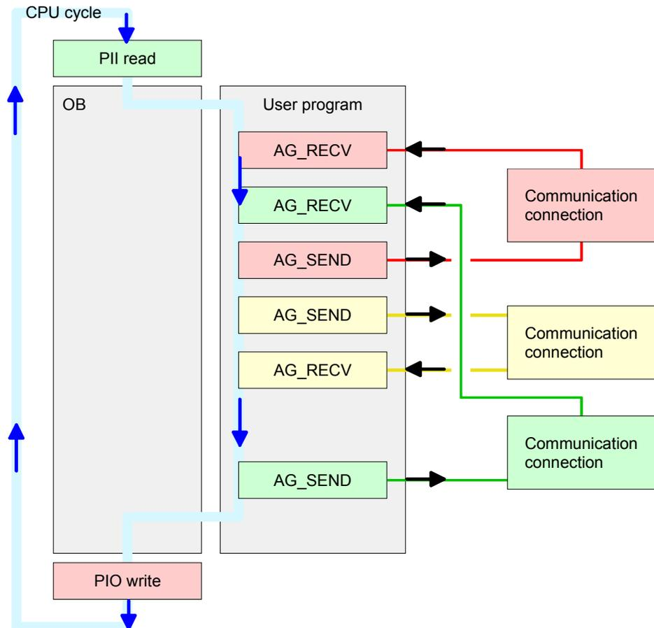
The FC blocks with concerning communication connection are summarized by color. Here you may also see that your user application may consist of any number of blocks. This allows you to send or receive data (with AG\_SEND res. AG\_RECV) event or program driven at any wanted point within the CPU cycle.
