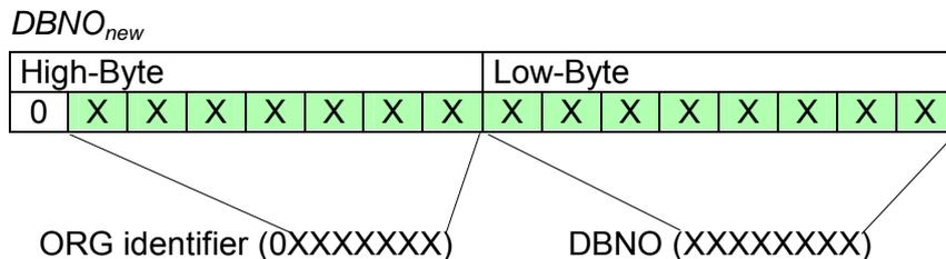
If the highest bit of the ORG identifier is set, the Low-Byte of DBNO<sub>new</sub> is defined via DBNO and the High-Byte of DBNO<sub>new</sub> via ORG identifier, where the highest bit of the ORG identifier is eliminated.
