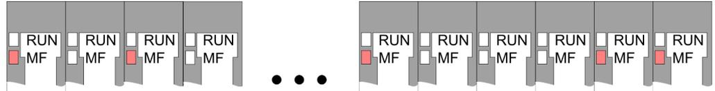
**Behaviour:** After PowerON the RUN LED of each module is off and the MF LED of each module is sporadically on.
