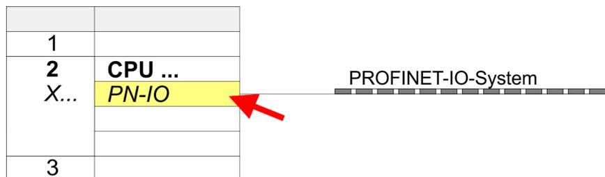
The PROFINET interface of the PROFINET IO controller is parameterized with PN-IO, the port with Port 1. In the following these parameters for PN-IO and Port 1 are described.
