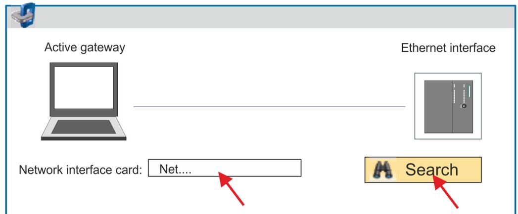
6. Select the according network interface card, which is connected to the Ethernet PG/OP channel and click at *'Search'* to determine the via MAC address reachable device.
