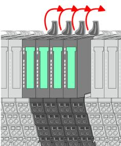
4. ➤ Turn all the locking lever of the module group to be exchanged upwards.
