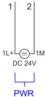
The CPU has an integrated power supply. The power supply has to be provided with DC 24V. Via the power supply not only the internal electronic of the CPU is provided with voltage, but also the electronic from the integrated IO modules and the sensor output. The power supply is protected against polarity inversion and over current.
