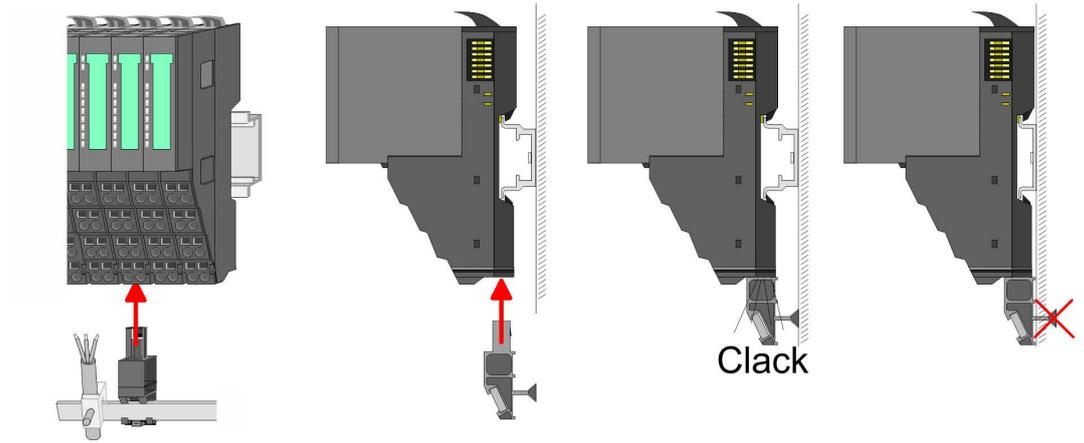
3. Attach the cables with the accordingly stripped cable screen and fix it by the shield clamp with the shield bus.
