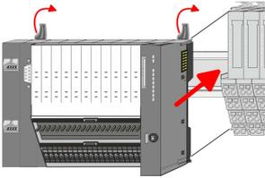
5. ➤ To mount the CPU put it to the periphery module and push it, guided by the stripes, to the mounting rail.
