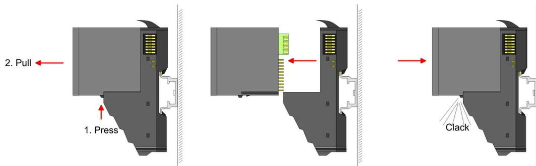
2. For the exchange of a electronic module, the electronic module may be pulled forward after pressing the unlocking lever at the lower side of the module.
