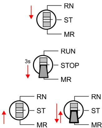
1. ➔ Your CPU must be in STOP mode. For this switch the operating mode switch of the CPU to STOP.
