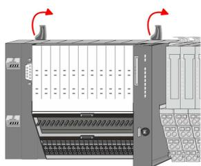
2. ➤ Turn all the locking lever of the CPU to be exchanged upwards.
