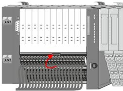
➤ Put the connector on the bottom edge and push it, as shown in the figure, with a rotation upwards into the release lever until it engages.
