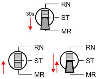
**2.** → Push the operating mode switch down to position MR for 30 seconds. Here the ST LED blinks. After a few seconds the ST LED changes to static light. Now the ST LED changes between static light and blinking. Start here to count the static light of the ST LED.
