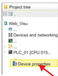
3. Via 'Device properties > WebVisu configuration' you can specify the port, the *WebVisu* can be accessed and upload SSL certificates. Please note that only SSL certificates in PEM format are supported.
