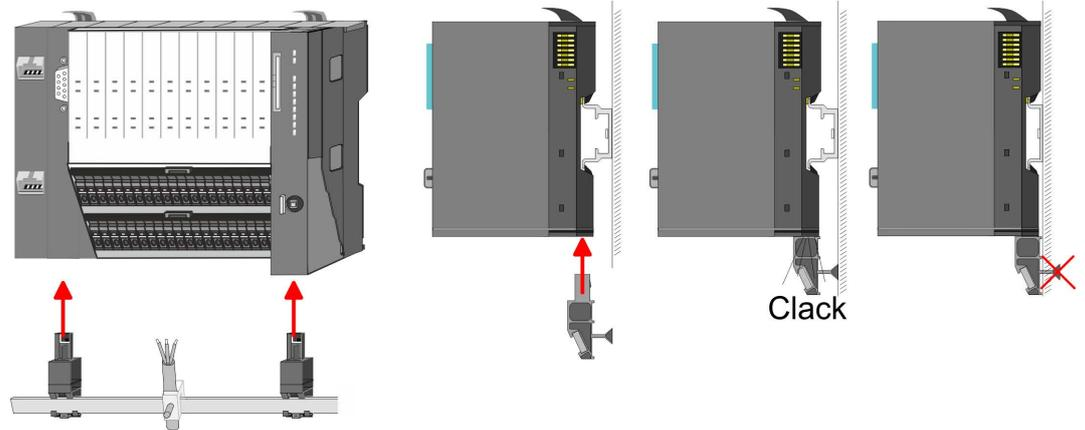
3. ➔ Attach the cables with the accordingly stripped cable screen and fix it by the shield clamp with the shield bus.
