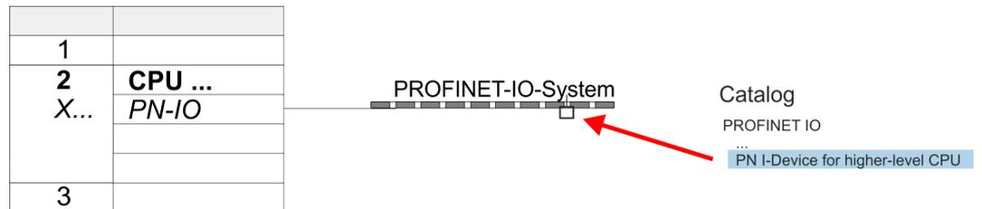
3. ➤ Open the properties dialog by double-clicking 'PN-I-Device' and enter at 'device name' the previously noted name of the VIPA I-Device.
