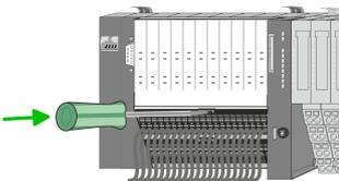
By means of a screwdriver there is the possibility to remove the connectors e.g. for module exchange with a fix wiring. For this each connector has a release lever centrally on its top side. Unlocking takes place by the following proceeding:
