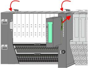
7. ➤ Plug again the electronic module, which you have removed before. For installation plug the electronic module guided by the strips at the lower side until this engages to the terminal module.
