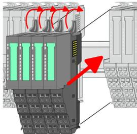
7. ➤ To mount the module group put it to the gap between the both modules and push it, guided by the stripes at both sides, to the mounting rail.
