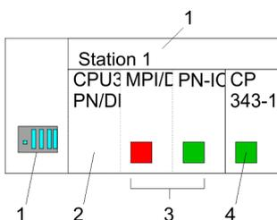
You receive the following graphical display for every PLC station and their component. By selecting the single components, the context menu offers you several functions:
