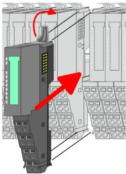
7. ➤ To mount the module put it to the gap between the both modules and push it, guided by the stripes at both sides, to the mounting rail.
