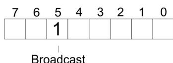
A request can be directed to a certain slave ore be send to all slaves as broadcast message. For the identification of a broadcast message you have to set bit 5 to 1 in the ADR byte. Here the slave addr. (bit 0 ... 4) is ignored. In opposite to a "normal" send command, the broadcast does not require a telegram evaluation via FC/SFC 218 SER\_RCV. Only write commands may be sent as broadcast.
