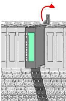
4. Turn the locking lever of the module to be exchanged upwards.
