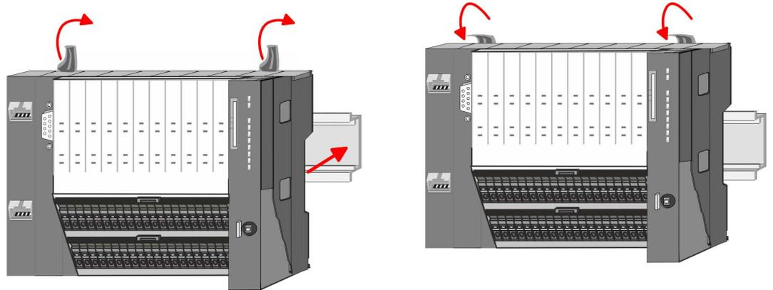
2. Turn the locking lever upwards, place the CPU at the mounting rail and turn the lever downward.
