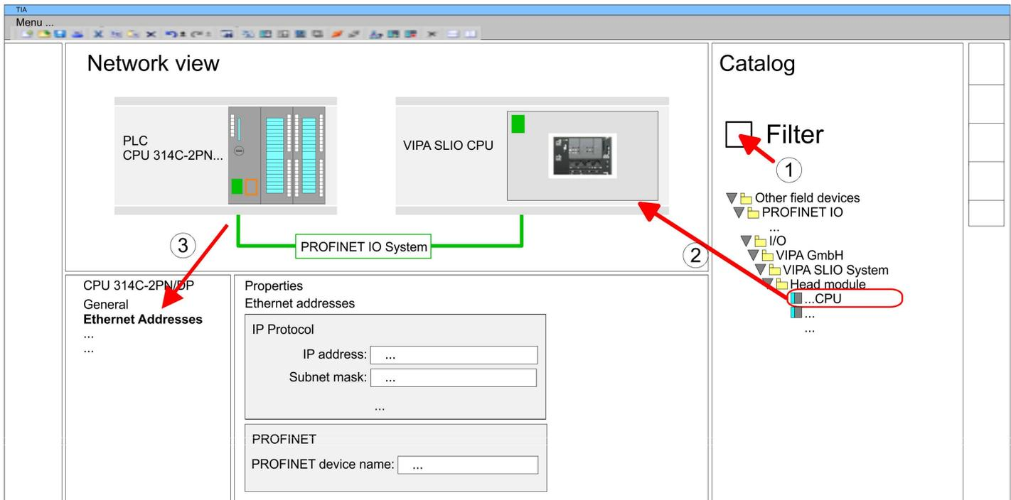
5. ➤ Select in the *Network view* the IO device 'VIPA SLIO CPU...' and switch to the *Device overview*.
