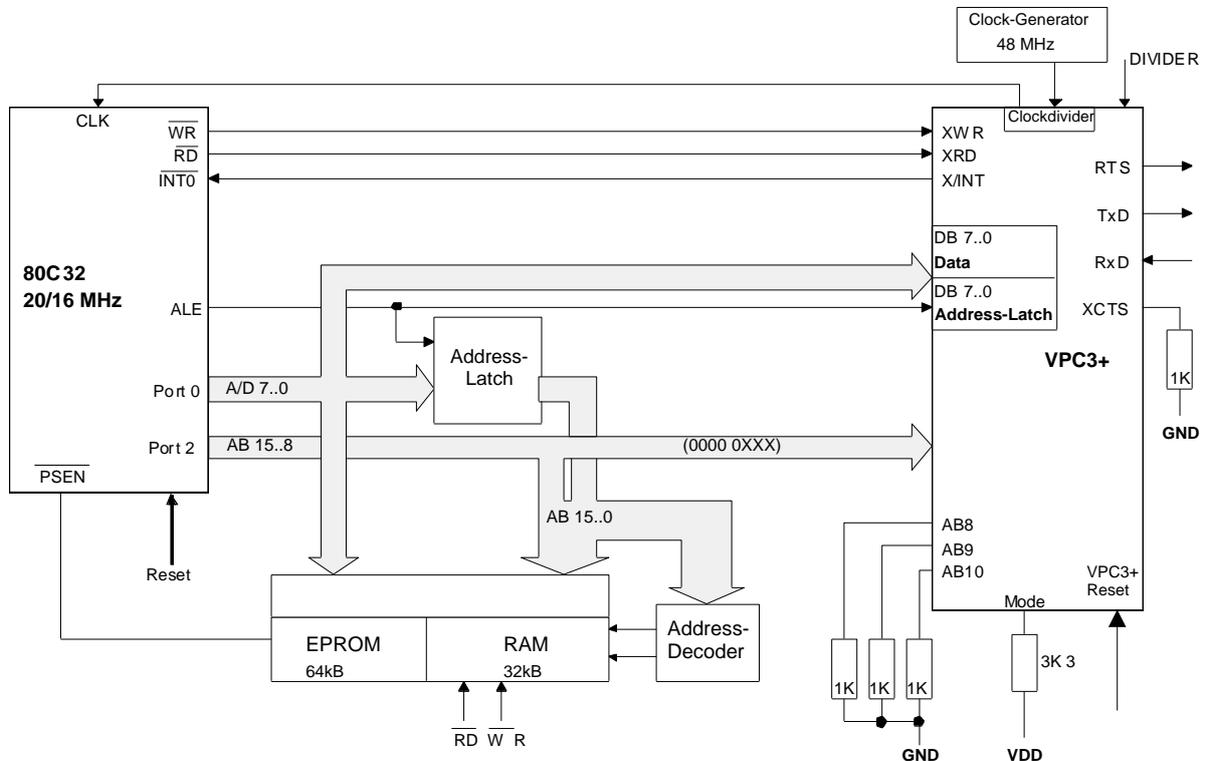
Figure 8-4: 80C32 System with External Memory
