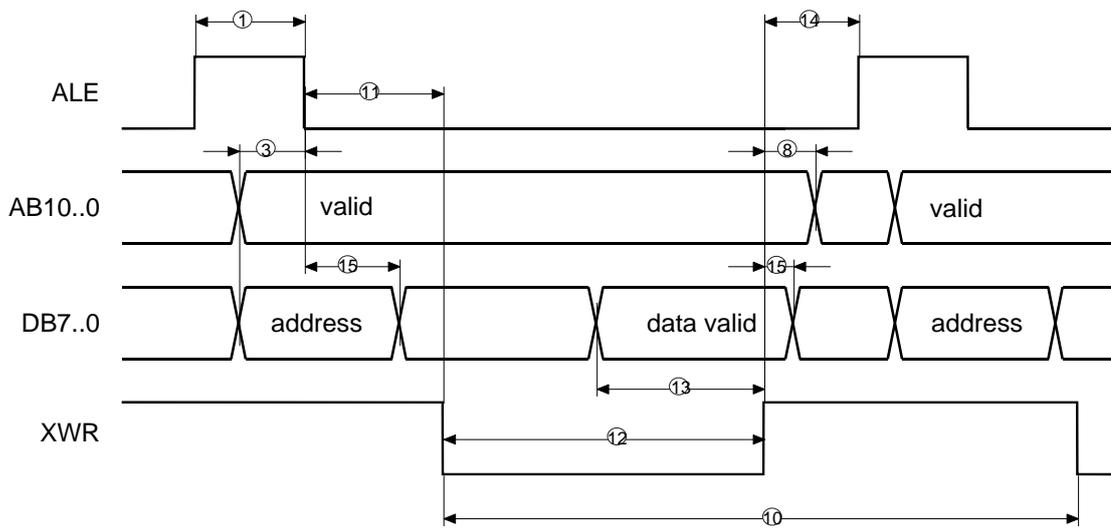
Figure 10-10: Synchronous Intel Mode, WRITE (XRD = 1)
