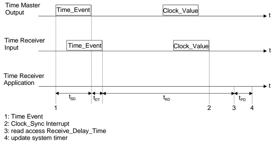
Figure 7-20: clock synchronization mechanism
