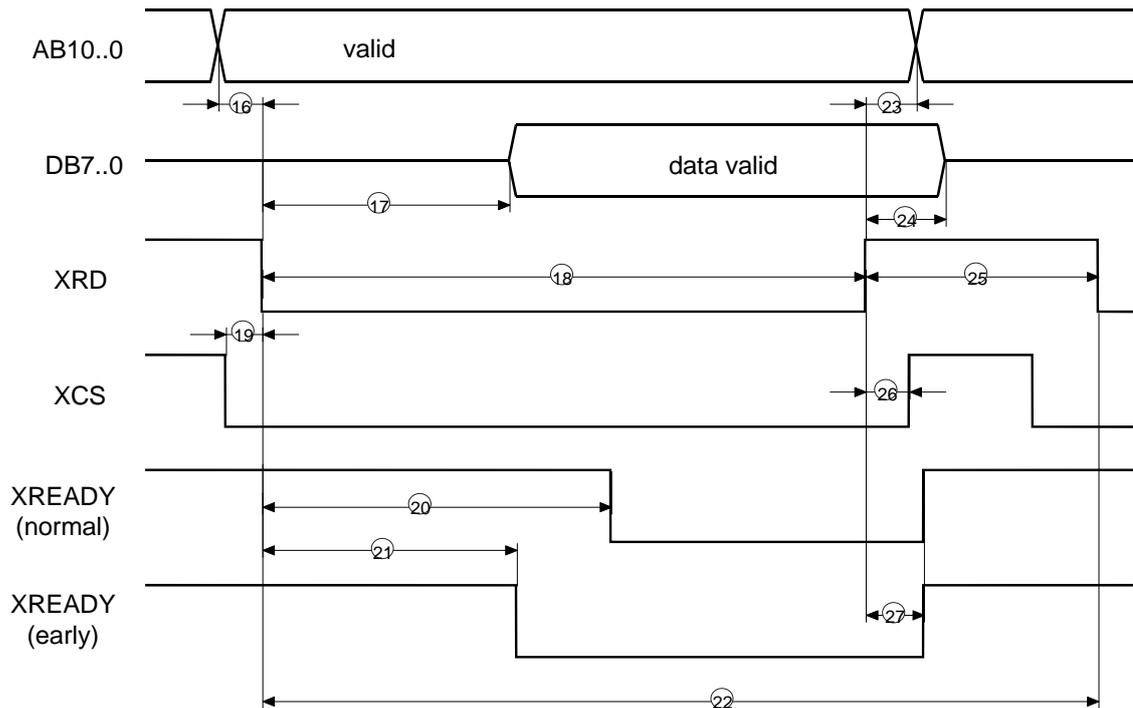
Figure 10-12: Asynchronous Intel Mode, READ (XWR = 1)
