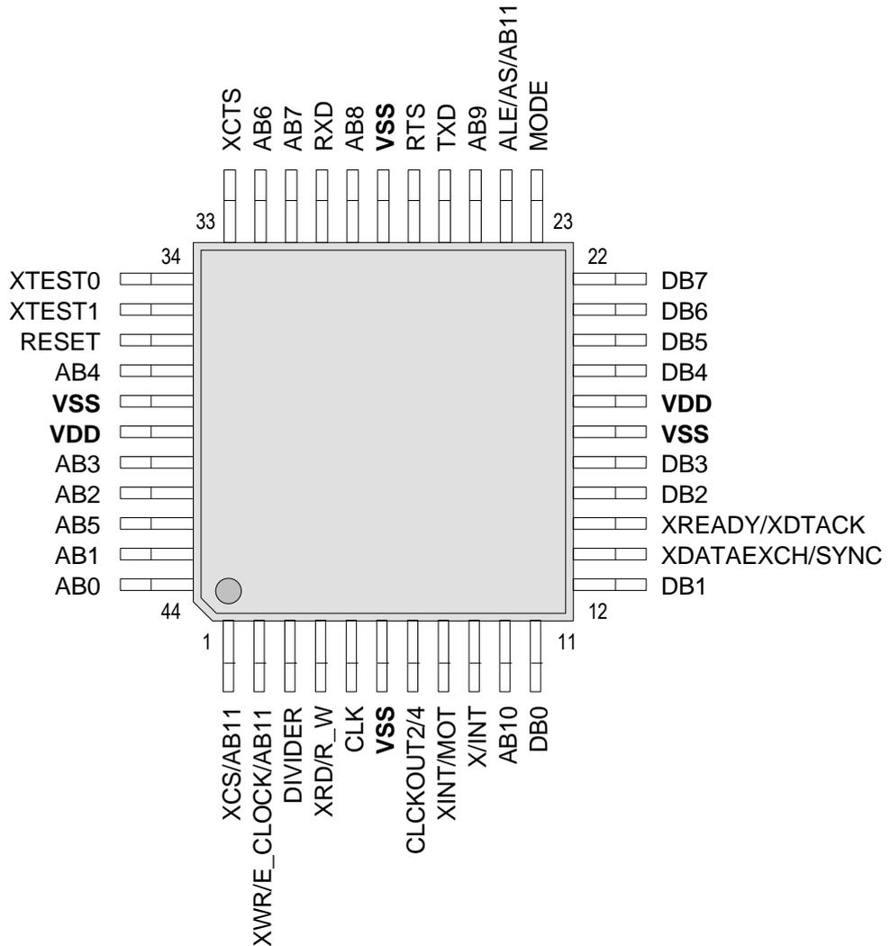
Figure 3-3: VPC3+C Pinout
