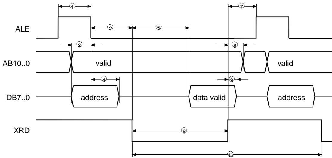
Figure 10-9: Synchronous Intel Mode, READ (XWR = 1)
