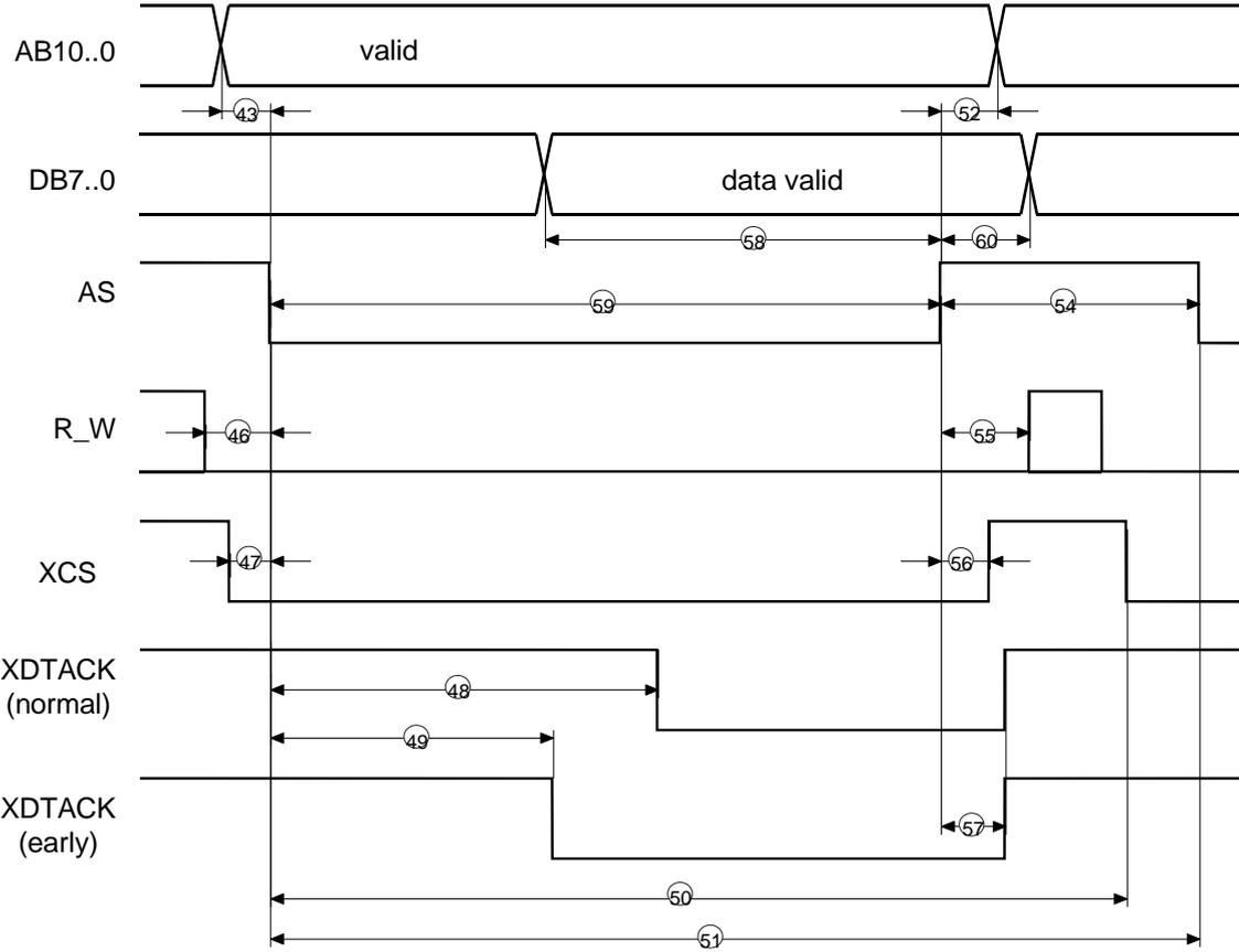
Figure 10-19: Asynchronous Motorola Mode (WRITE)
