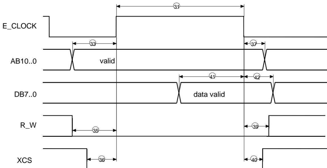
Figure 10-16: Synchronous Motorola-Mode, WRITE (AS = 1)
