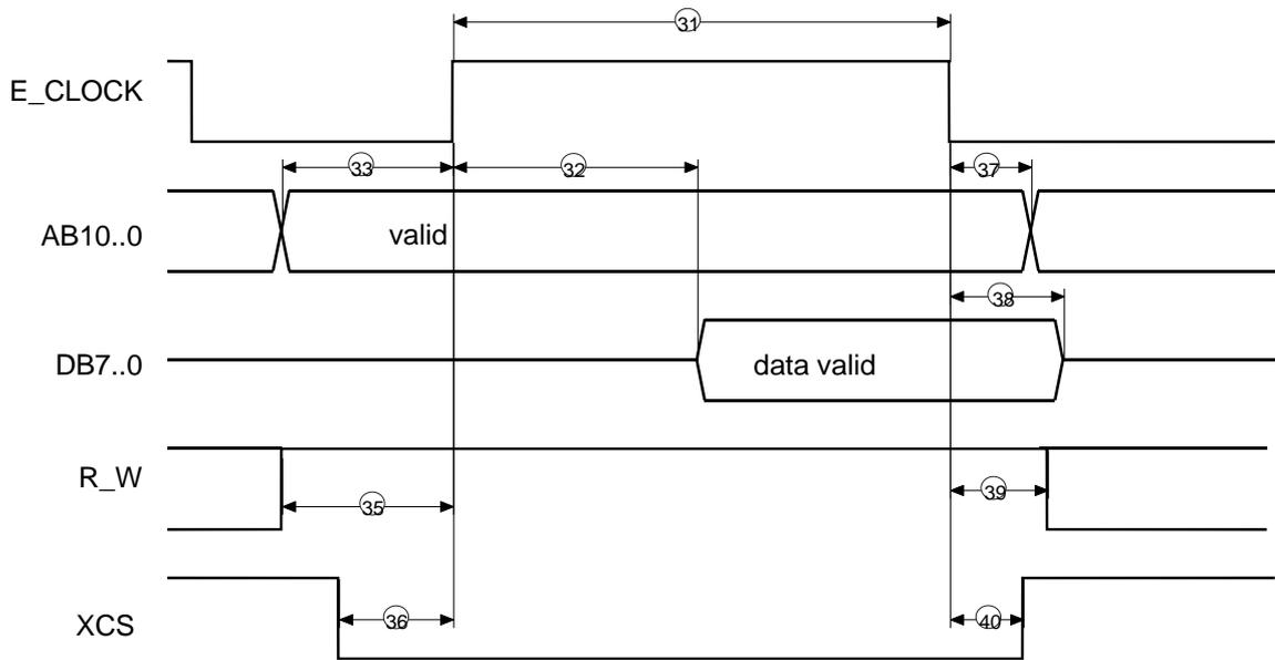
Figure 10-15: Synchronous Motorola-Mode, READ (AS = 1)
