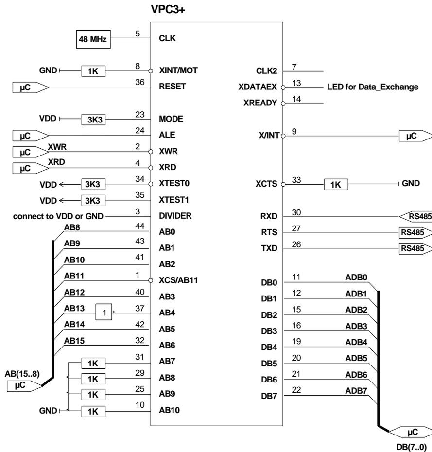
Figure 8-8: 80C32 Application in 4K Byte mode
