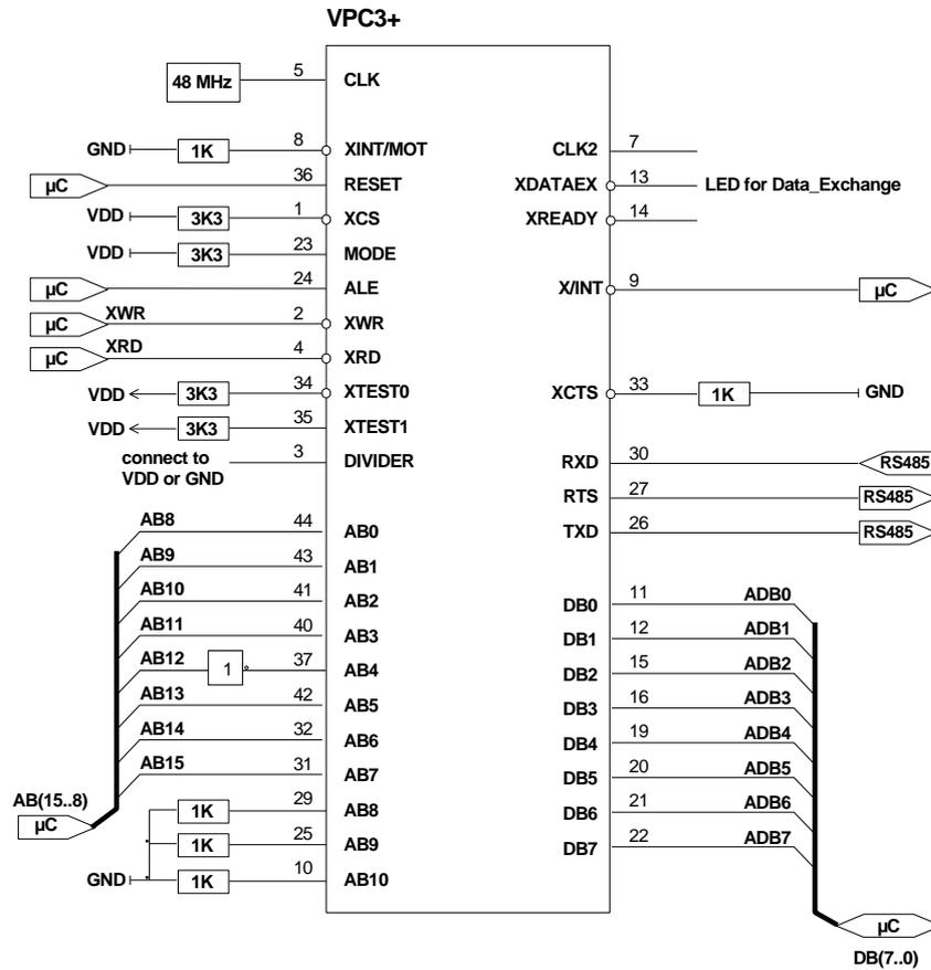
Figure 8-6: 80C32 Application in 2K Byte mode
