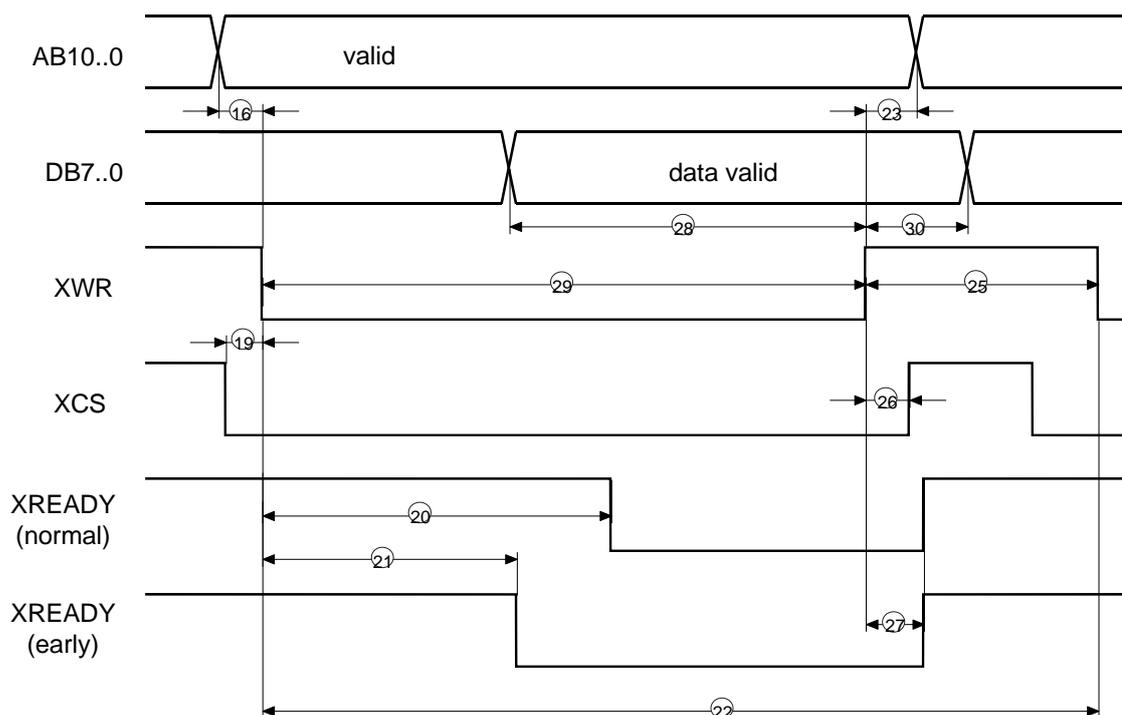
Figure 10-13: Asynchronous Intel Mode, WRITE (XRD = 1)
