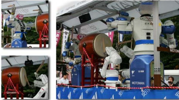
Taiko drum robot installation (2 DA20 robots and 2 HP3L robots)
